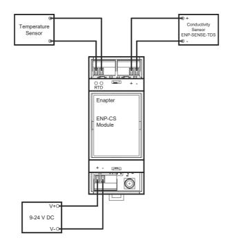
Note: 1 Amp Circuit Breaker recommended to use on power line for the ENP-CS Module.
