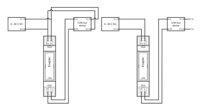
Note: 1 Amp Circuit Breaker recommended to use on power line for the ENP-CAN Module.
