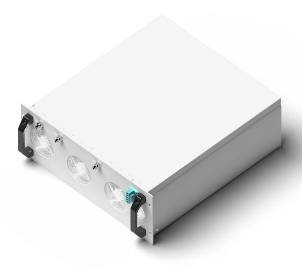
Enapter's dryer is a hybrid temperature/pressure swing adsorption system that comprises of cartridges filled with a highly adsorbent material. The dryer is maintenance-free. During operation, one cartridge catches the humidity from the hydrogen gas stream of the electrolyser, while the other cartridge is heated and regenerated. The dryer is rackmountable in a standard 19" cabinet.
